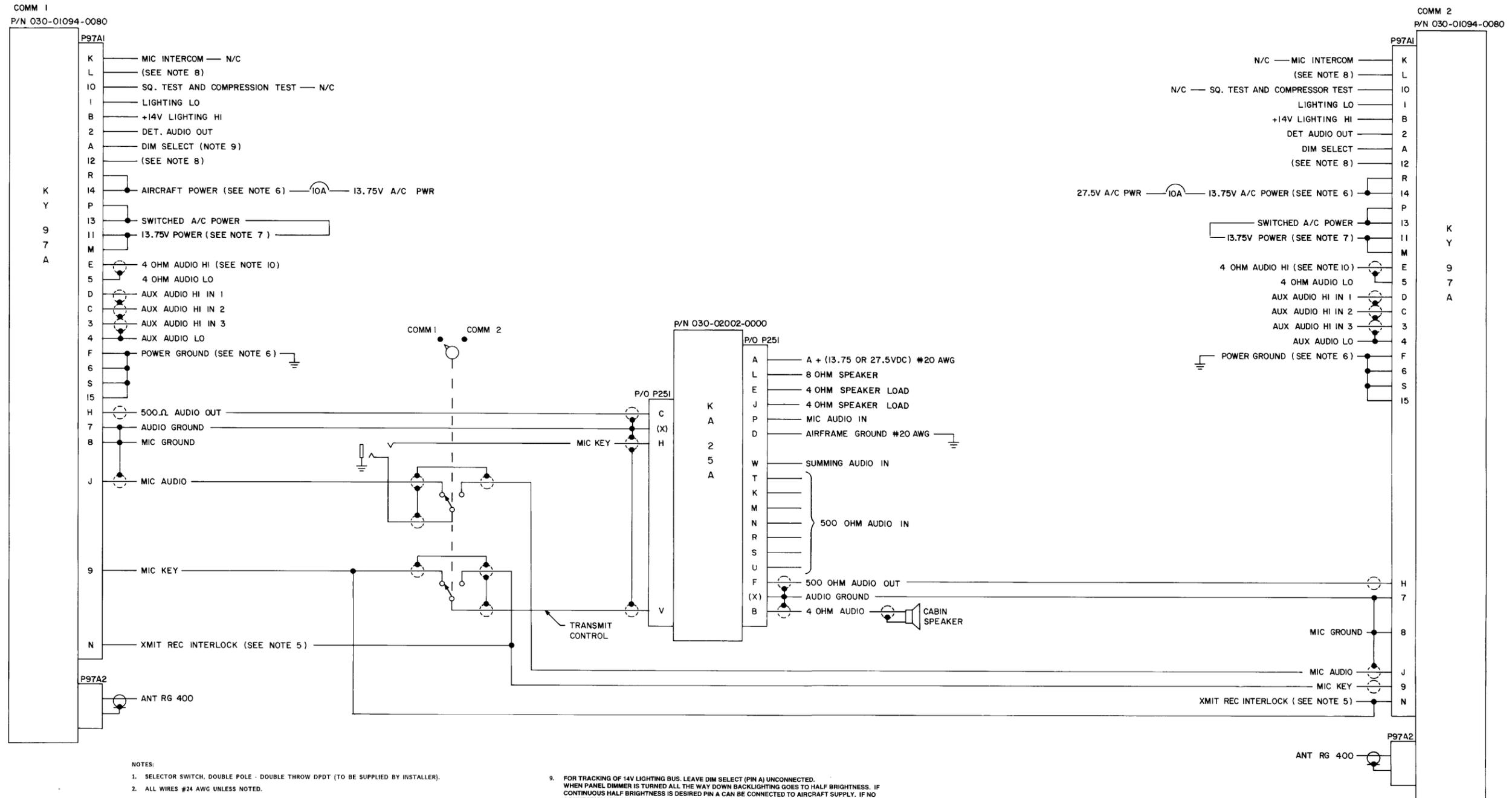
FIGURE 2-13 Dual KY 97A with KA 25A interconnect
