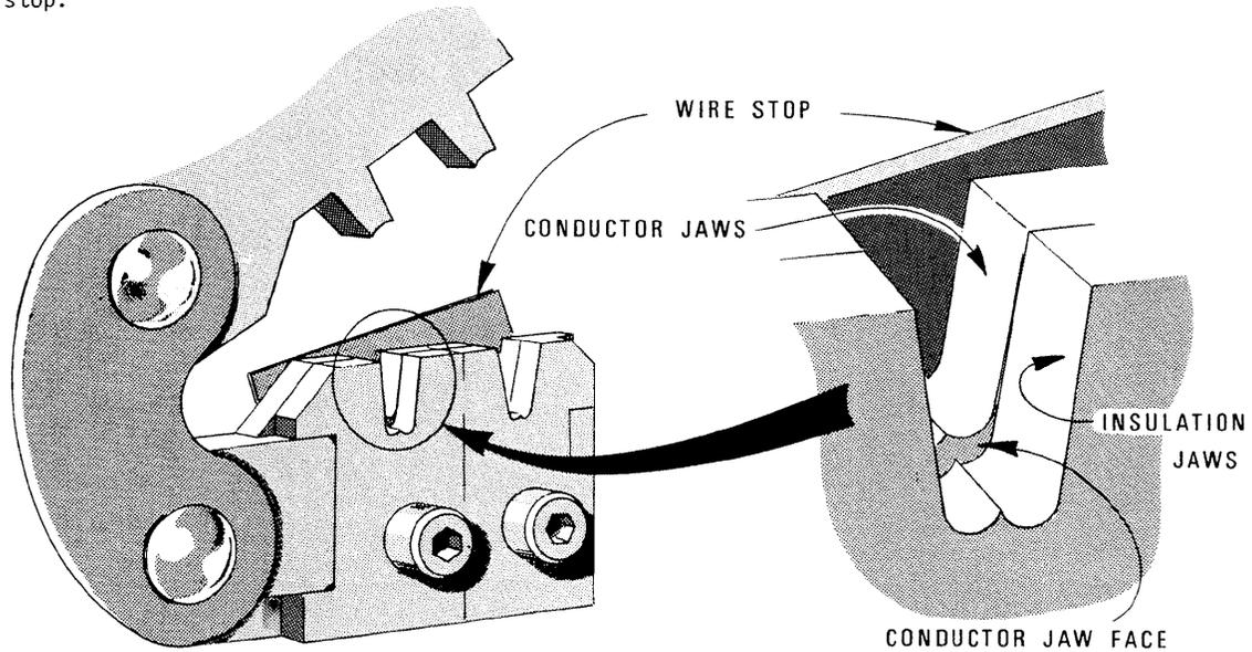
Squeeze the handles until the crimp jaws close and the ratchet releases.
