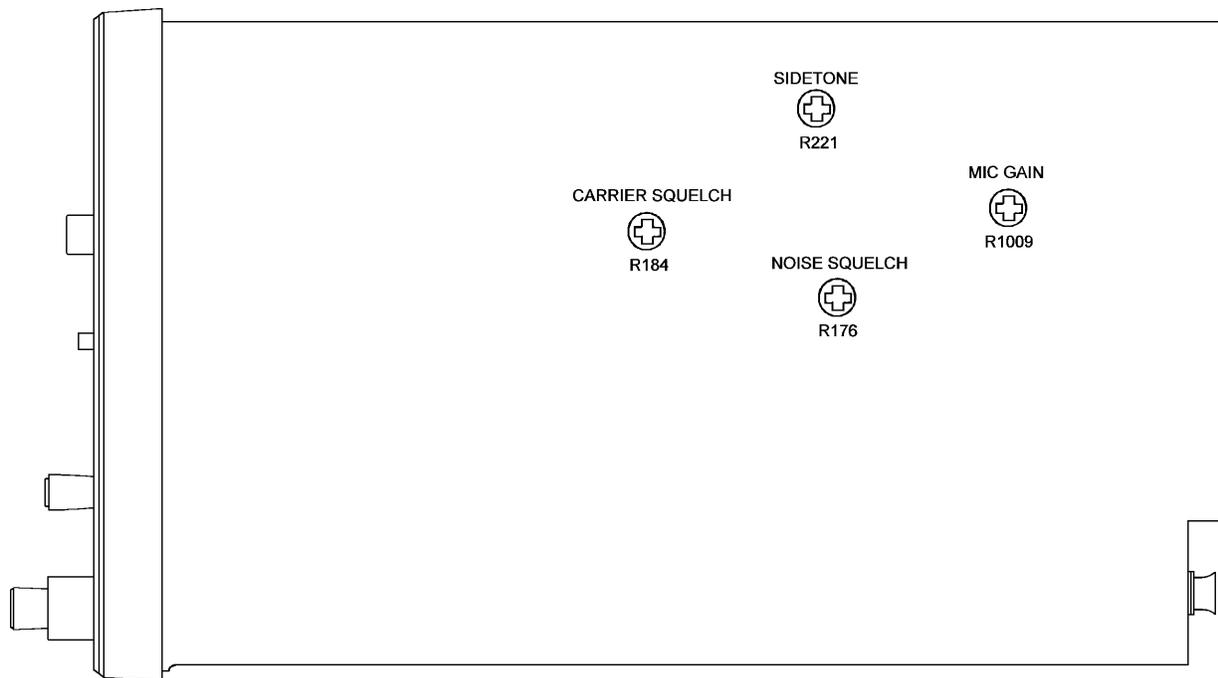
FIGURE 2-1 KY 96A, KY 97A Cover-On Adjustments
