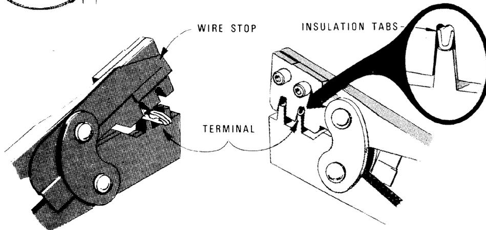
Terminal is in correct position when insulation tabs are flush with outside face of crimp jaws.
