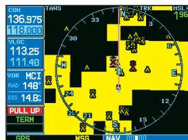
Terrain awareness meets tower avoidance in Garmin's GNS 530. In addition to aural and visual terrain alerts, an obstacles database helps pilots see and avoid towering man-made structures as well.
