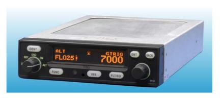
The TT31 is a power efficient, inexpensive, Mode S general aviation transponder. The TT31 meets the European elementary surveillance requirements, and fits the same mounting tray as the popular KT76A transponder, making it ideal for both new and retrofit installations.
