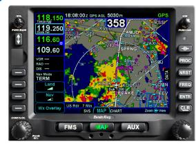
The AeroNav 900 is a full-featured GPS/FMS/ NAV/COM with hybrid touchscreen/physicalknobs, wireless connectivity, 3-D synthetic vision and internal ADAHRS built right in.
