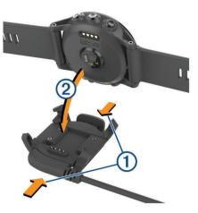
4 With the contacts aligned, place the device into the cradle ② and release the arms to hold the device in place.
