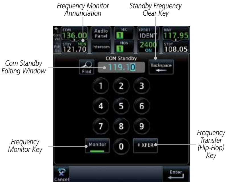
Figure 3-24 Com Frequency Monitoring
