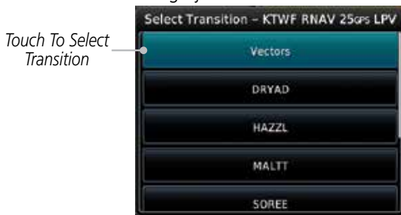
Figure 6-15 Select Approach Transition
