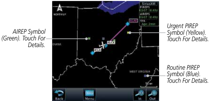
Figure 12-40 Weather Display With AIREP/PIREP Information Active
