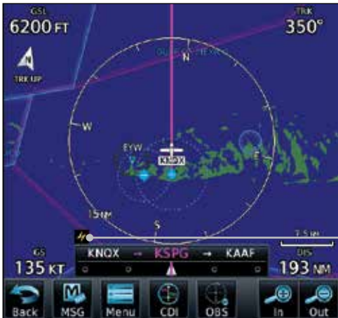
Figure 9-10 Map Menu StormScope Map Overlay On Selection
