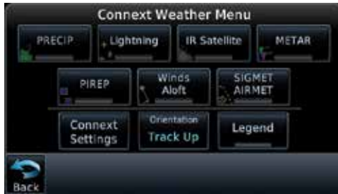
Figure 12-70 Select Connex Weather
