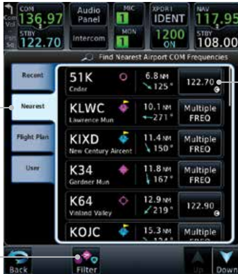
Figure 3-6 Com Nearest Airport Frequency
