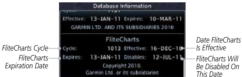
Figure 7-24 System Status Database Information for FliteCharts
