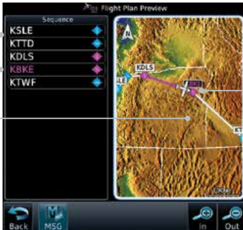
Figure 4-46 Active Flight Plan Preview
