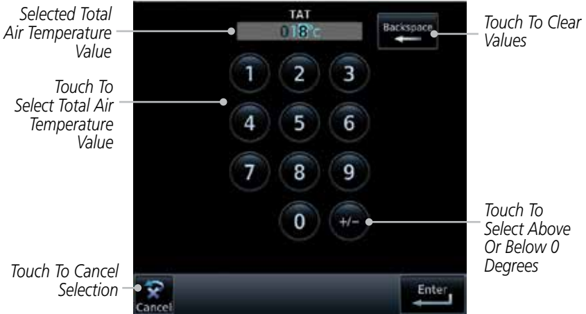
Figure 15-41 Select Total Air Temperature Value
