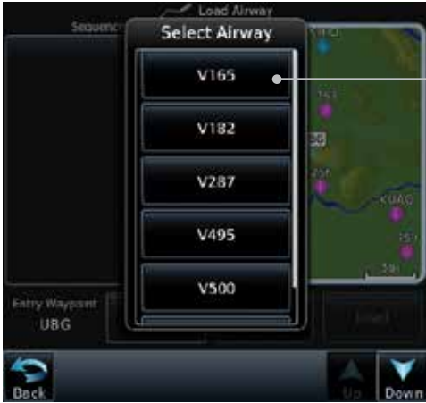
Figure 4-19 Select an Airway from the List
