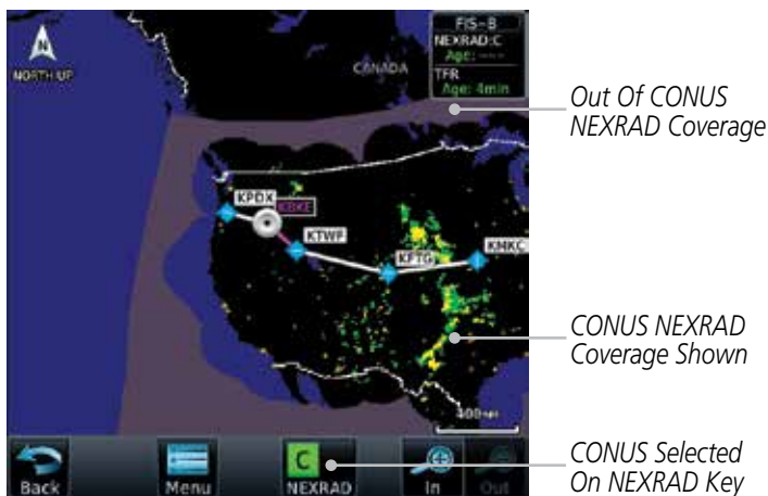
Figure 12-95 Weather Page With CONUS Displayed
