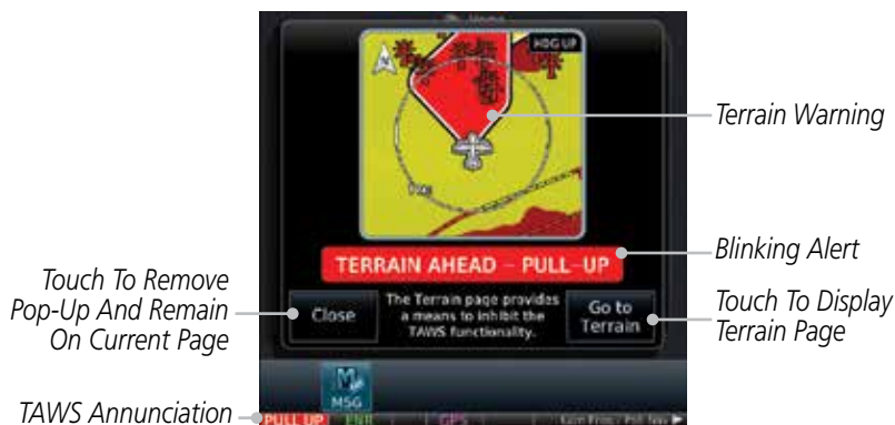
Figure 11-32 Terrain Alert Pop-Up
