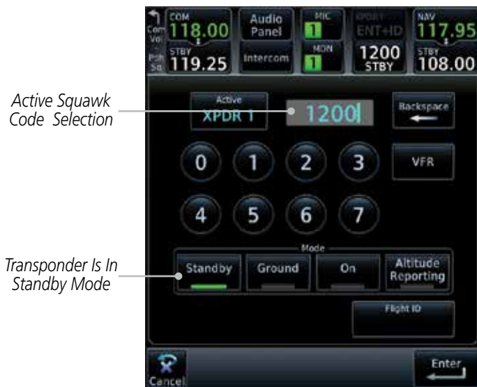
Figure 2-8 XPDR Squawk Code Selection Display
