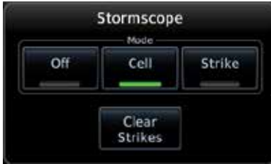
Figure 9-9 Map Menu StormScope Map Overlay Selection
