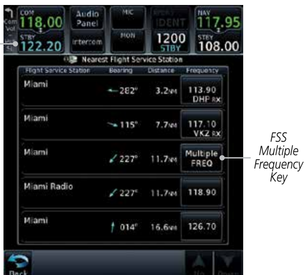
Figure 13-23 Selected FSS Frequency From List
