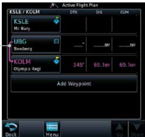
Figure 4-17 Active Flight Plan with VOR Entry Wpt
