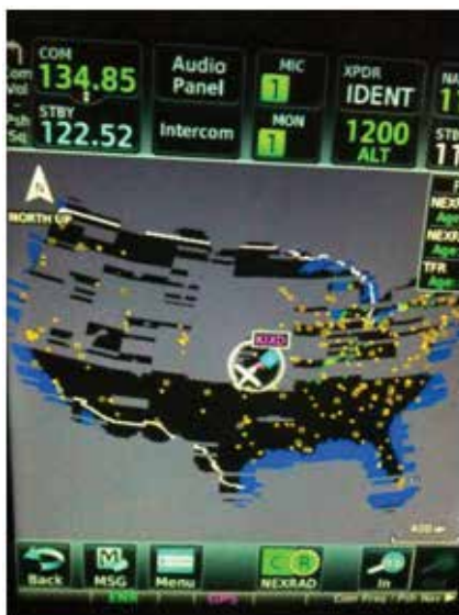
Figure 12-94 Example of Areas Where FIS-B Reception Is Unavailable
