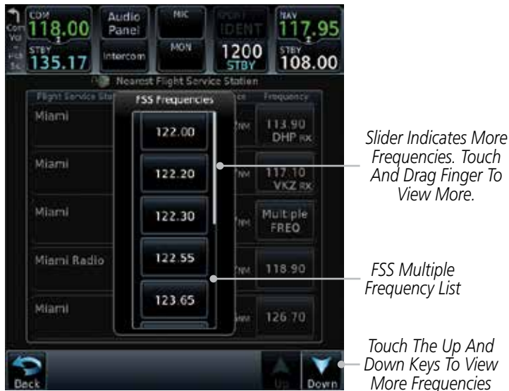
Figure 13-22 Nearest FSS Multiple Frequency List
