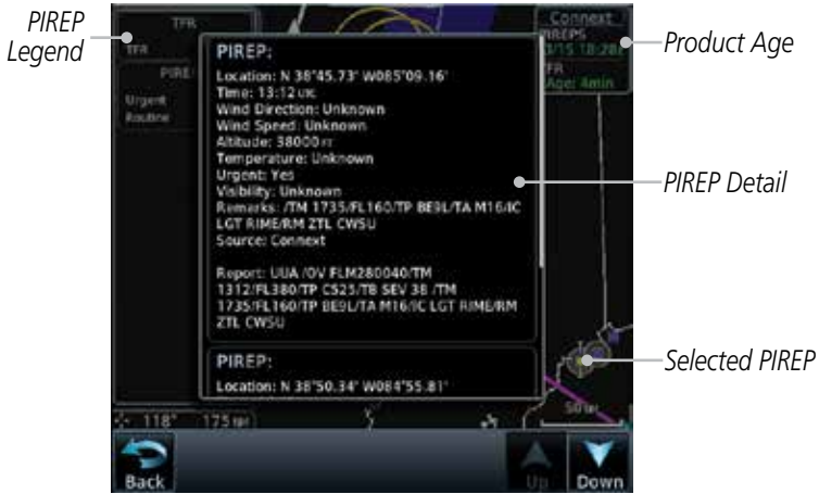
Figure 12-84 Connex Weather - PIREPs
