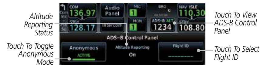
Figure 2-10 ADS-B Control Panel
