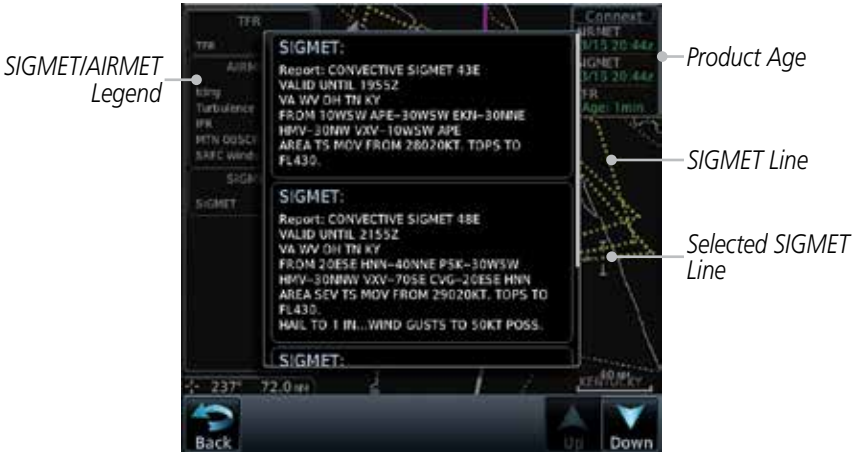
Figure 12-88 Connex Weather Page - AIRMETS/SIGMETs
