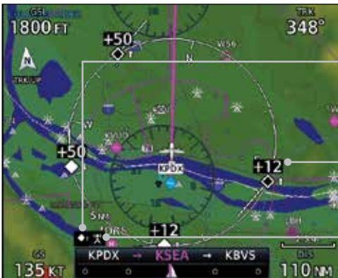
Figure 9-12 Map Menu Traffic Map Overlay On Selection
