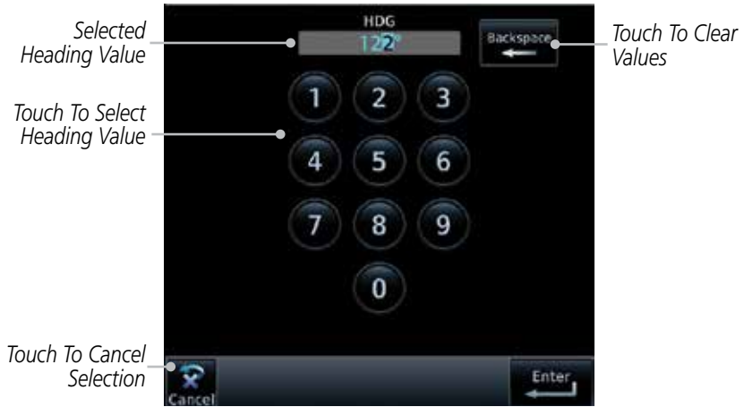
Figure 15-43 Select Heading Value
