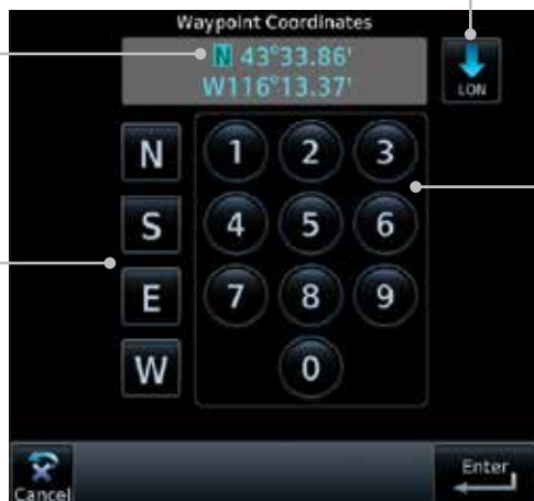
Figure 8-24 Lat/Lon Coordinate Selection
