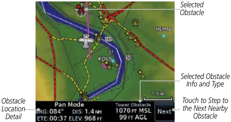
Figure 9-22 Point Obstacle Detail
