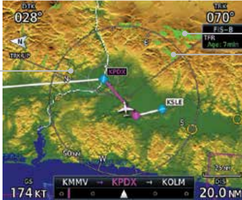
Figure 9-11 Map Menu Radar Map Overlay On Selection
