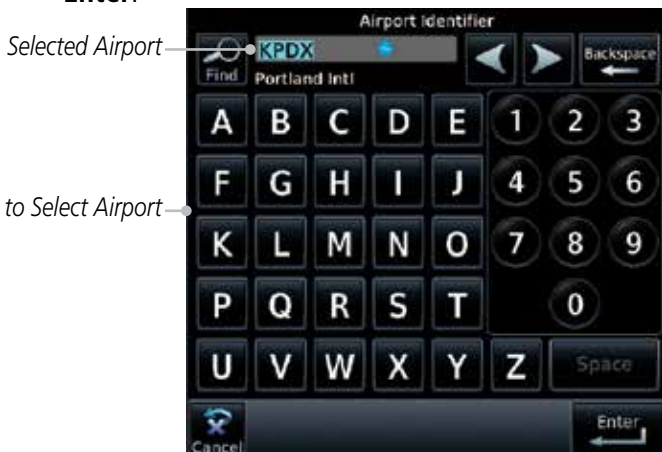
Figure 7-3 Airport Identifier Selection
