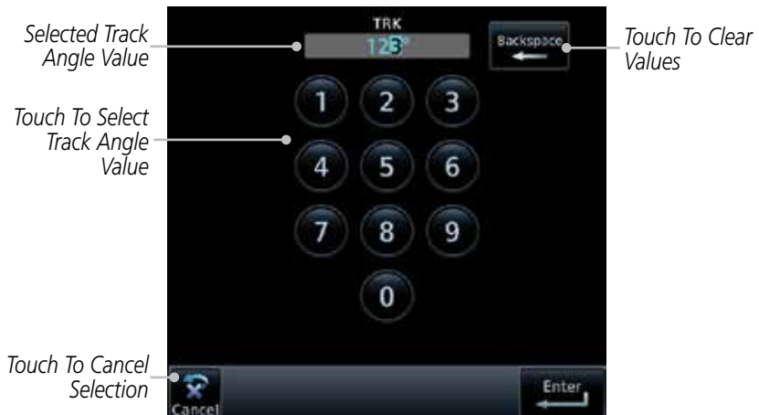
Figure 15-42 Select Track Angle Value
