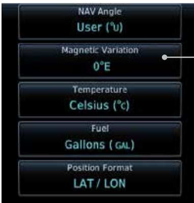
Figure 16-47 Magnetic Variation is Available for Editing
