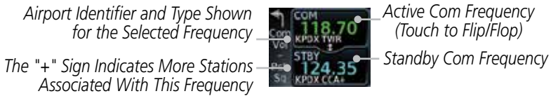
Figure 1-21 Com Radio Frequency Windows (Touch Active to Flip/Flop)
