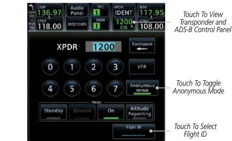
Figure 2-11 ADS-B/Transponder Control Panel
