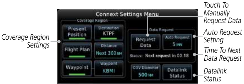
Figure 12-72 Connex Settings Menu
