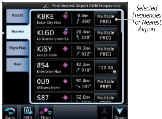
Figure 3-8 Com Nearest Airport Frequency
