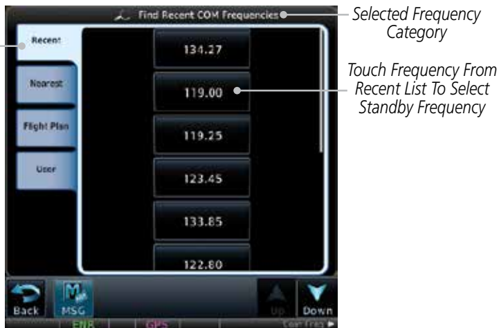
Figure 3-7 Recent Com Frequency List
