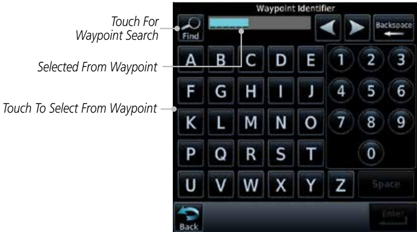
Figure 15-15 Selecting a From Waypoint
