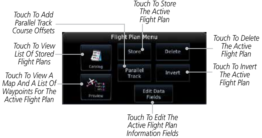
Figure 4-25 Flight Plan Menu
