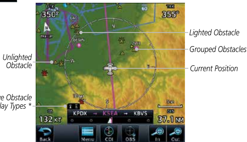
Figure 9-21 Navigation Map Point Obstacles
