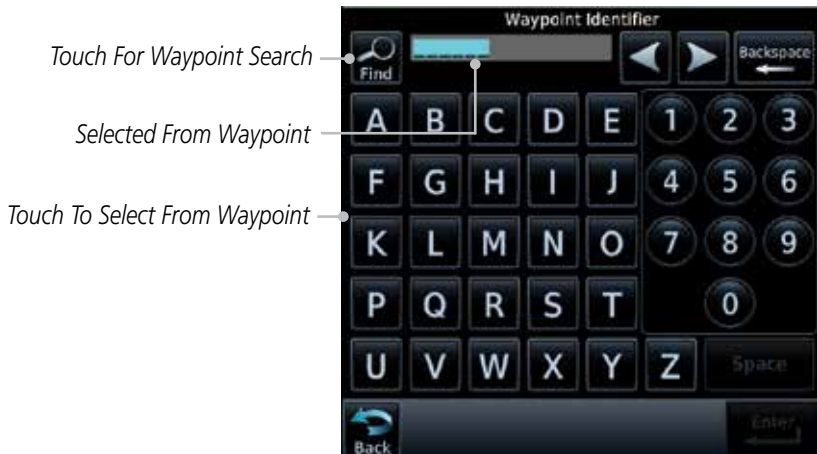
Figure 15-28 Selecting the From Waypoint
