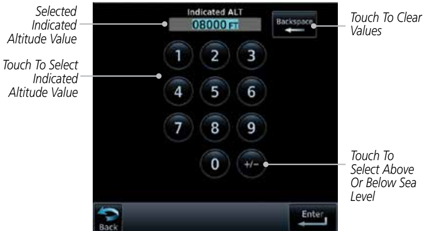
Figure 15-38 Select Indicated Altitude Value
