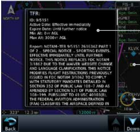
Figure 12-100 FIS-B TFR Detail
