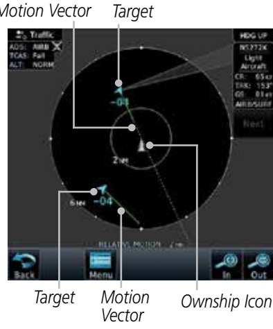
Figure 10-16 Comparison of Absolute and Relative Motion Vectors With a Two Targets
