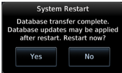
Figure 16-9 System Restart - Step 1
