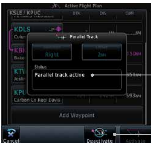
Figure 4-31 Deactivating Parallel Track
