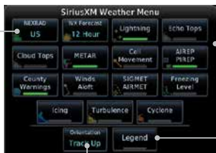
Figure 12-5 SiriusXM Weather Menu
