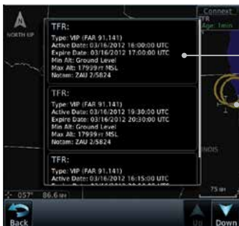
Figure 12-79 ConnexT TFR Detail
