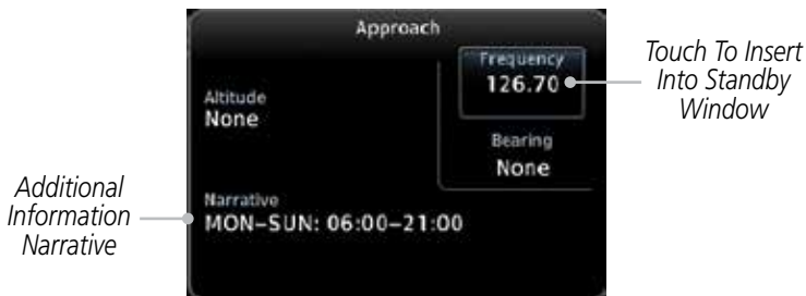
Figure 3-12 More Frequency Detail
