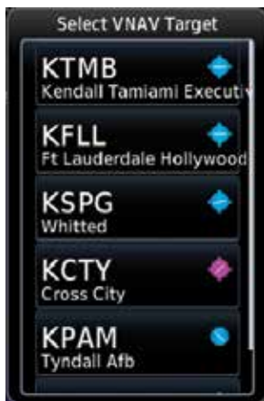
Figure 15-9 Select VNAV Target Waypoint List
