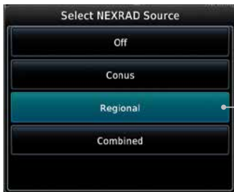
Figure 12-98 NEXRAD Source Selection
