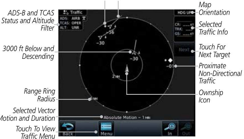
Figure 10-13 Absolute Motion (White Vectors)
