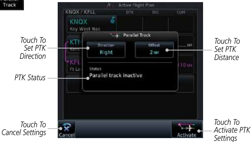
Figure 4-29 Parallel Track Selection
