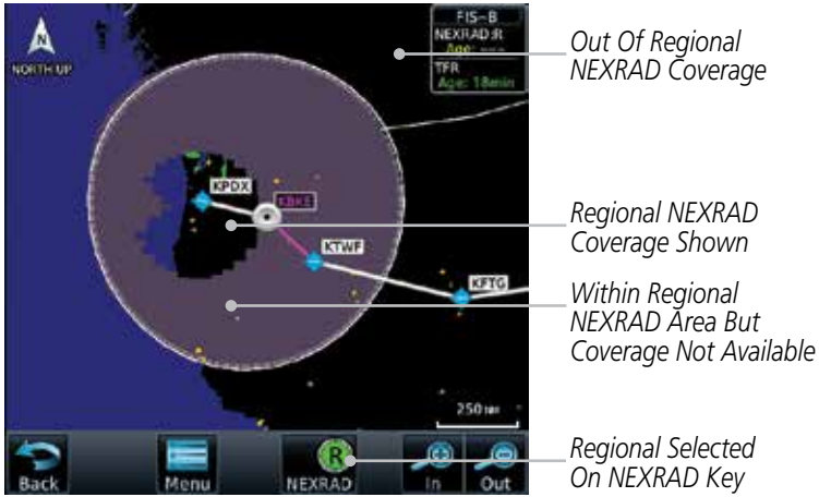
Figure 12-96 Weather Page With Regional NEXRAD Displayed
