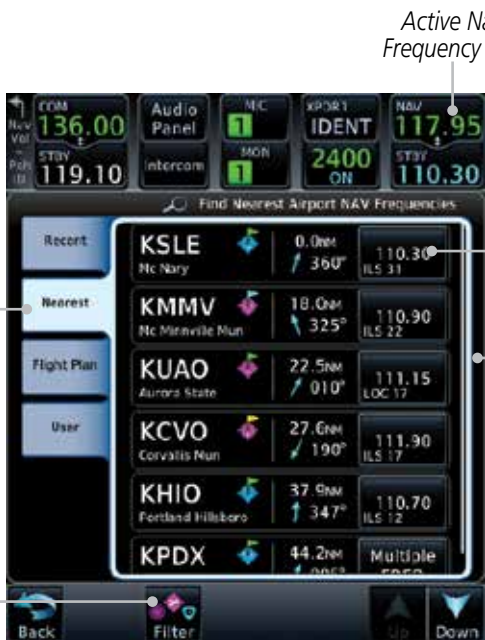
Figure 3-28 Nearest Airport Nav Frequency
