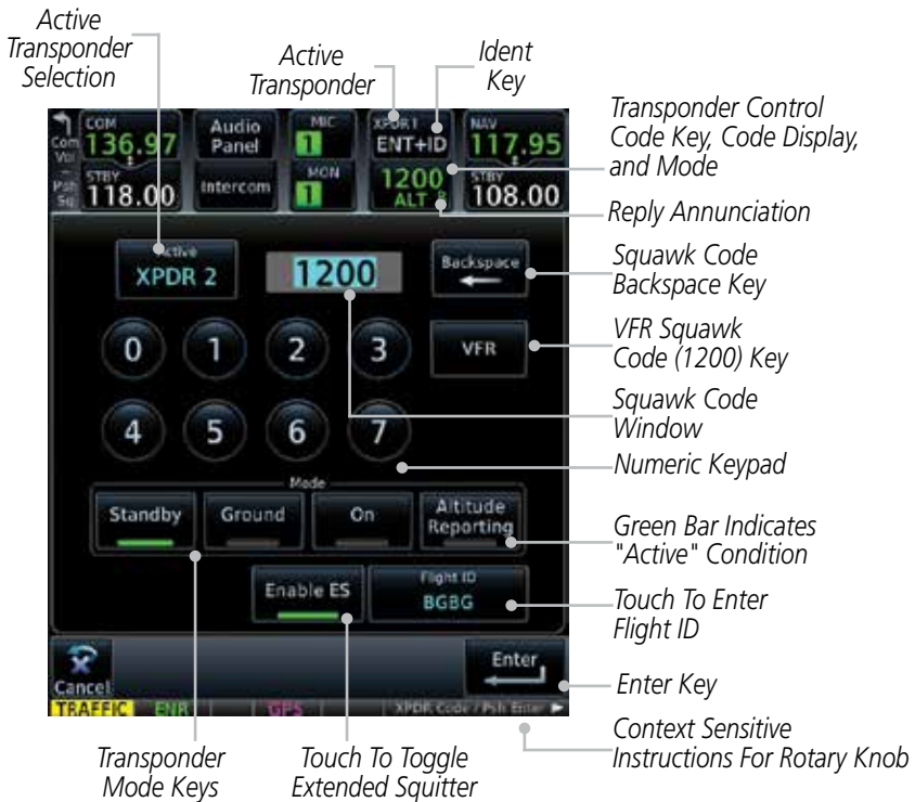
Figure 2-1 XPDR Control Display
