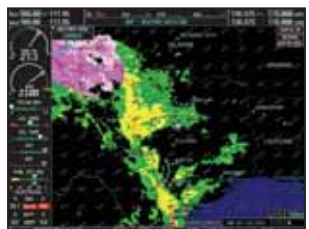
G1000 - Precipitation types along with winds aloft allows pilot to avoid hazardous conditions and forecast future movement along the route of flight
